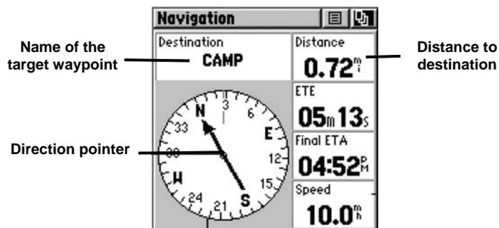
4. When the distance to the target is less than 3 m (10 ft) and arrow becomes unstable, stop and try to locate the waypoint. Measure how many steps are left to reach the waypoint and record your observations in the table below.
