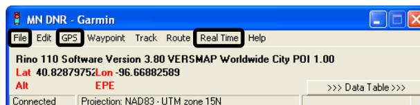
Go to GPS > Set Baud Rate > 4800 (NMEA mode) to set up for real time tracking. Go to Real Time > START Real time tracking. In the real time window choose Point and click Load File and save as an ArcView Shapefile (projected) to start saving real time data to a shapefile in ArcMap. Specify the path as given by your instructor.
