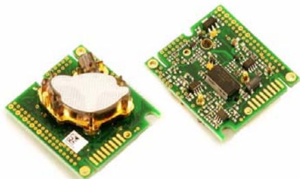
SenseAir's CO 2 Engine® K30 CO 2 Sensor
