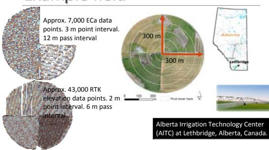
Approx. 7,000 ECa data points. 3 m point interval. 12 m pass interval.
