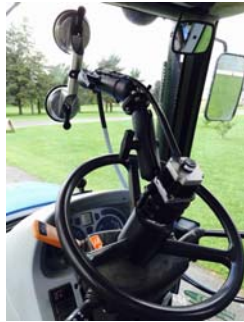
Steering apparatus mounted to the front window of the tractor.
