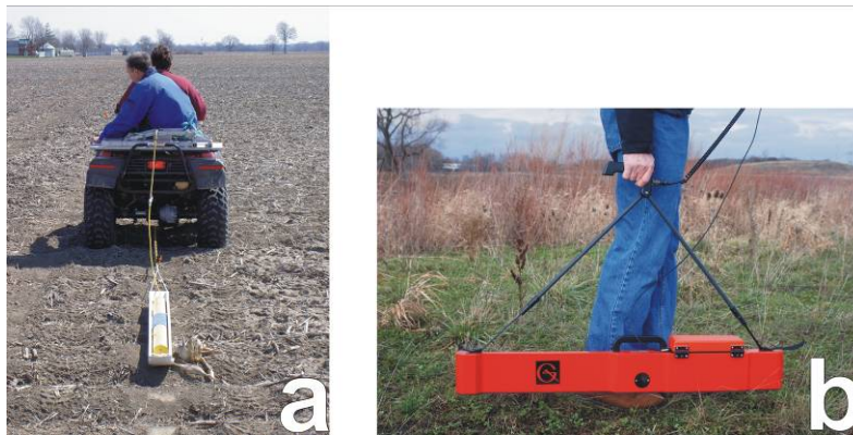
Figure 2. Examples of ground conductivity meters used in agroecosystem settings; (a) DUALEM-1S (Dualem Inc., Milton, Ontario, Canada), and (b) EM38-MK2 (Geonics Limited, Mississauga, Ontario, Canada).
