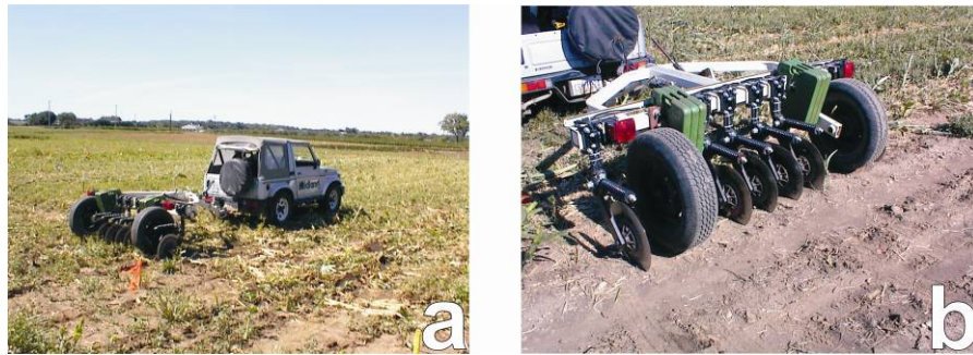
Figure 1. Example of a continuous measurement galvanic contact resistivity system; (a) Veris 3100 Soil EC Mapping System (Veris Technologies, Salina, Kansas, U.S.A.) and (b) close-up of steel coulters used for current and potential electrodes by the Veris 3100 Soil EC Mapping System.
