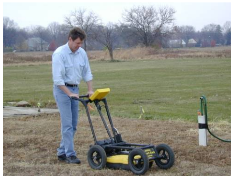
Figure 3. Example of GPR system (Sensors & Software Inc., Noggin plus with 250 MHz antennas - Mississauga, Ontario, Canada) being used to map buried agricultural drainage pipes.
