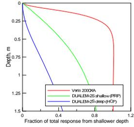
Because of variations in instrument response with depth, EC<sub>a</sub> is affected not only by soil variables (salinity, clay, water content, etc.) but also how they are layered in the profile
