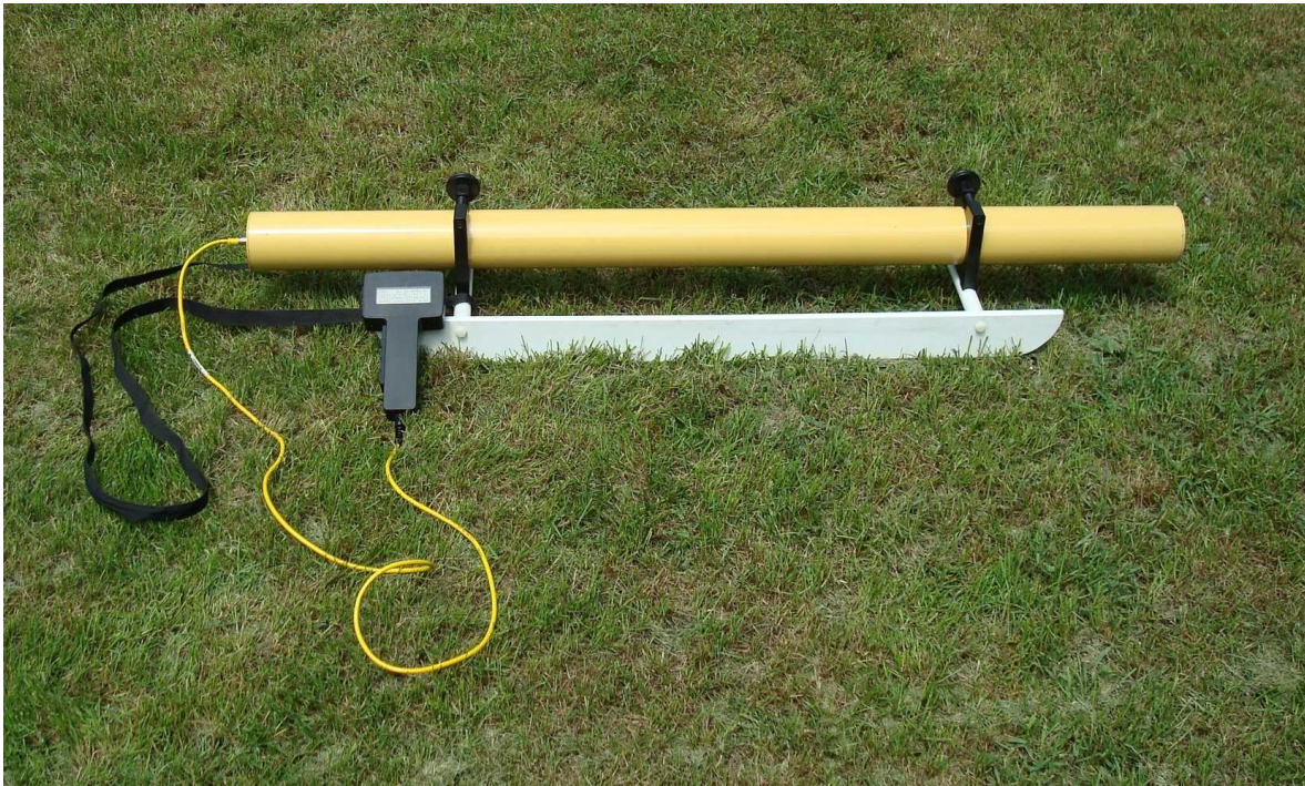
Figure 1: DUALEM-1 on sled.
