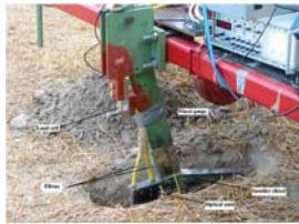
On-line multi-sensor platform (Mouazen, 2006)
